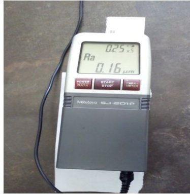
Fig 2: Mitutoyo surface roughness tester SJ-210
